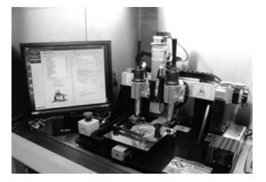
**Figure 3.** The NovoGen MMX Bioprinter has a footprint that enables it to fit into a standard biosafety cabinet. Features of the first-generation instrument include two dispensing heads, temperature control, automatic calibration, and a custom software interface for integrated experimental design and instrument control.
