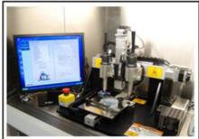
Figure 3. The NovoGen MMX Bioprinter has a footprint that enables it to fit into a standard biosafety cabinet.. Features of the first-generation instrument include two dispensing heads, temperature control, automatic calibration, and a custom software interface for integrated experimental design and instrument control.
